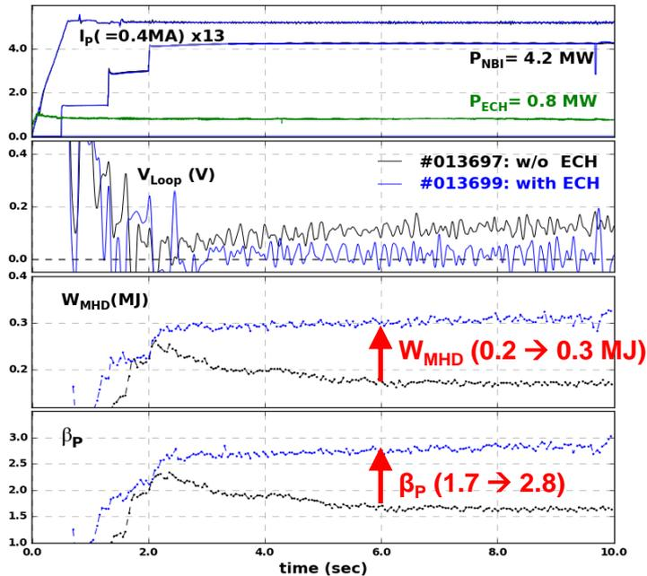
Stationary high beta discharge ( $\beta_N \sim \beta_p \sim 2.8$ ) at 0.4 MA, 3.9 MW NBI and 0.7 MW ECH
