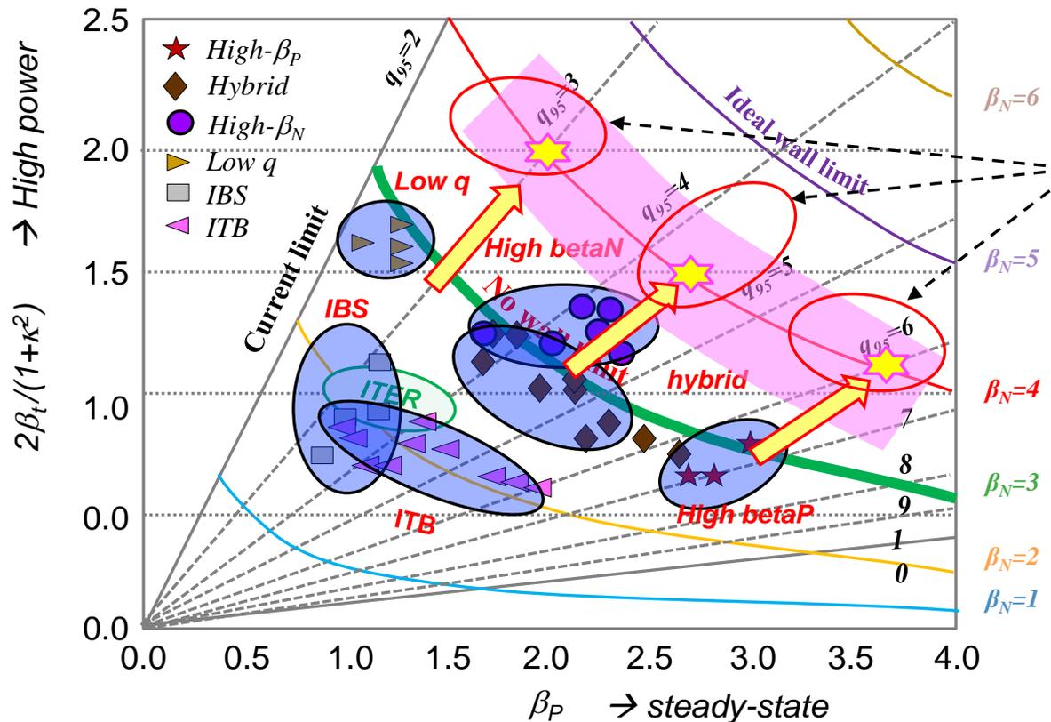
Extrapolation to high beta operation after heating upgrade based on 2017 experiments
